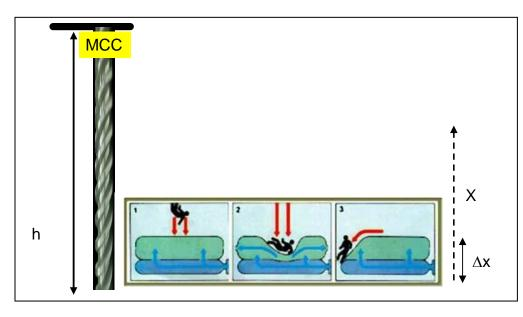
A testing system of cloths jump for building evacuation consists on a motor that automatically adjusts the jump height based on the X value of the rebound possible from the cushion.
